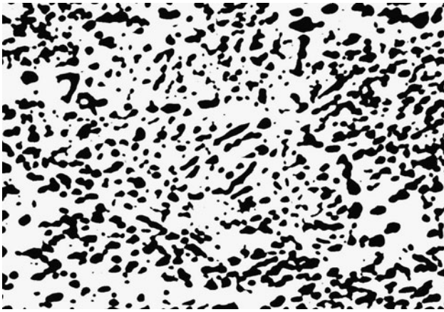
Fig. 5 Enhanced image showing only the areas of carbide particles in the 24% cold-rolled 50CrV4 steel after 6 h annealing at 720 °C
